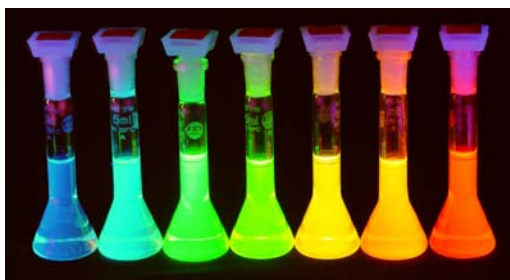
A series of CdSe based nanoparticles with growing size from left to right between 3 and 6 nm.
