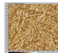
AFM picture of P3HT nanofibers:PCBM active layer
