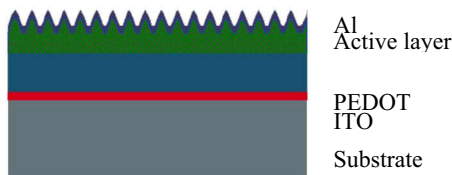
Figure 3: Cross-section of the patterned organic plastic solar cell
